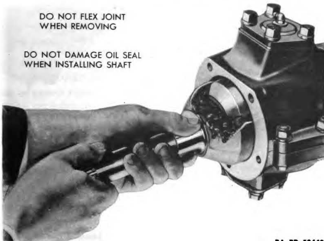
Figure 48—Removing Universal Drive Shaft
