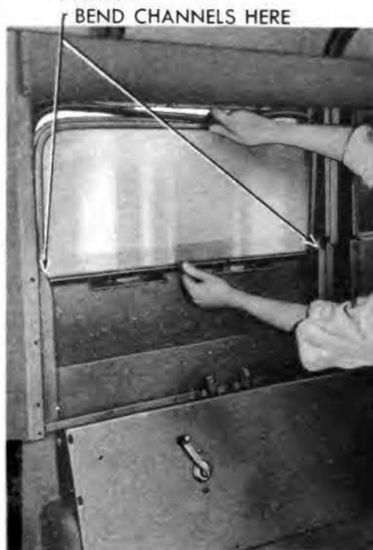
4—REMOVING SIDE WINDOW GLASS
