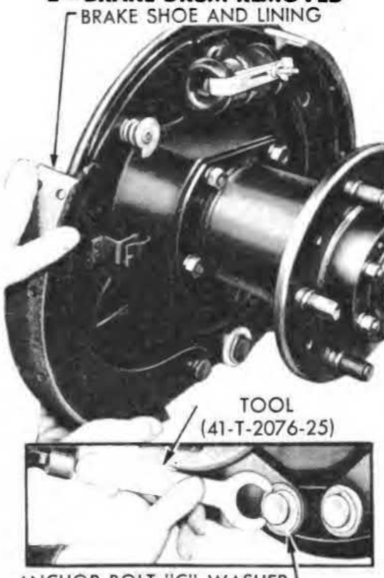
TOOL (41-T-2076-25) ANCHOR BOLT "C" WASHER 4—REMOVING BRAKE SHOE
