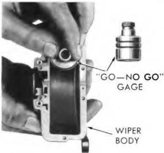
1—CHECKING WIPER BODY WITH "GO-NO GO" GAGE
