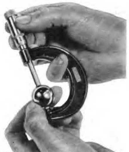
4—MEASURING DRIVE BALLS WITH MICROMETER
