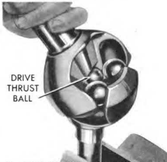
3—REMOVING OR INSTALLING UNIVERSAL DRIVE BALLS
