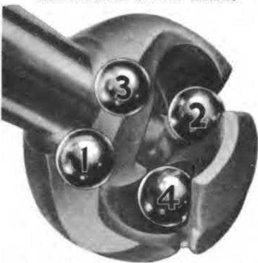
5—DRIVE BALL INSTALLATION DIAGRAM
