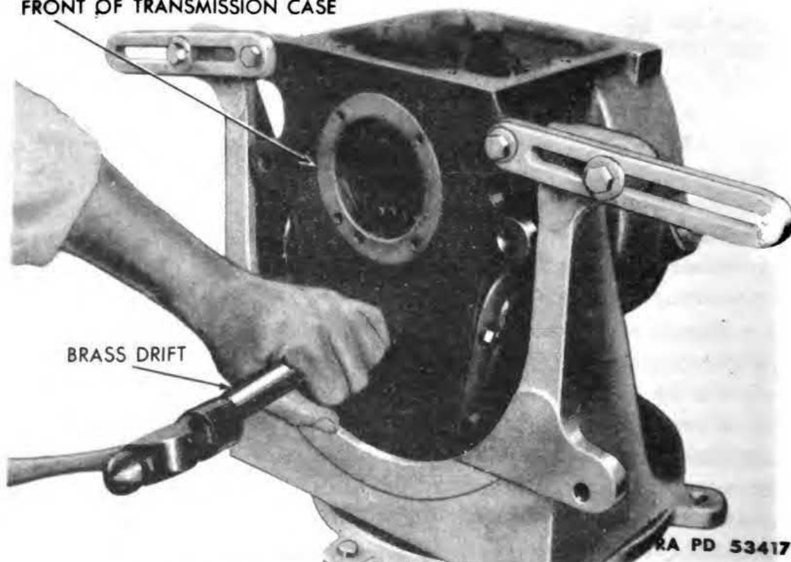
2—REMOVING TRANSMISSION COUNTERSHAFT
