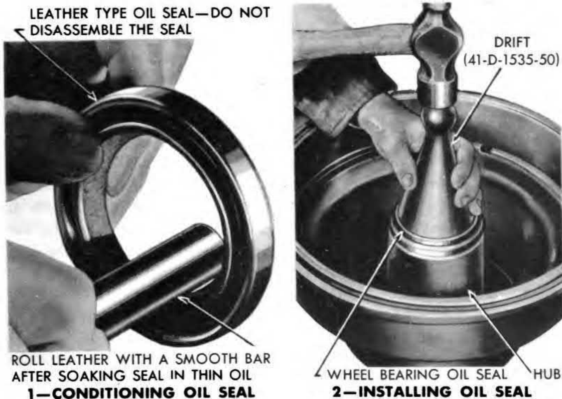
Figure 62—Conditioning and Installing Rear Wheel Bearing Oil Seal
