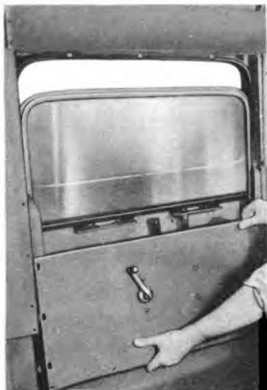
3—REMOVING SIDE WINDOW REGULATOR PANEL
