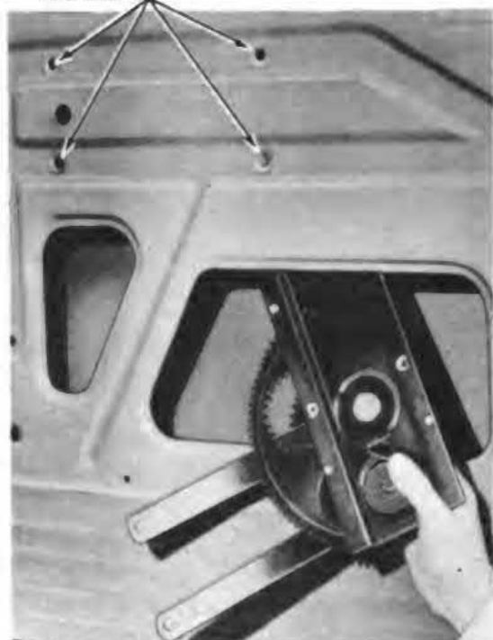
1—REMOVING DOOR WINDOW REGULATOR
