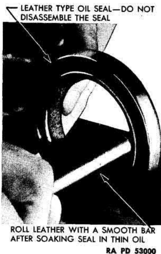
Figure 155—Conditioning Oil Seal
