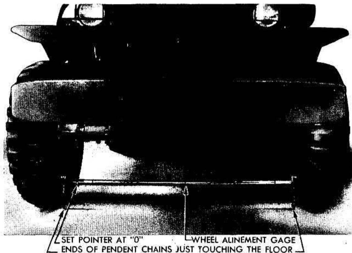
Figure 150—Front Wheel Toe-in Adjustment
